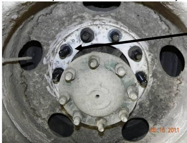
**Locate 1<sup>st</sup> stud clockwise from the valve stem; install the first anti-indexing sleeve. If everyone follows this procedure, you will have**
