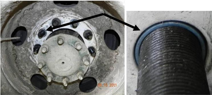
**WARNING:** Selecting an anti-indexing sleeve that is too long may damage the brake drum face and/or interfere with the nut's flange washer producing false or lower torque and clamp load, resulting in the wheel(s) loosening or separating from the vehicle causing; property damage, injury, even death.
